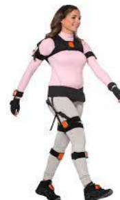
Fig. 2 – Sensor fastening structure on the player’s garment (3).
