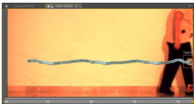
Fig. 2 – Using the system to follow the knee marker during one walk - screenshot from Adobe After Effects, where the element that captures the trajectory can be seen.
